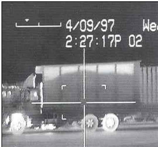
Figure 6: IRISystem Detecting Inoperable Brakes on the Vehicle
