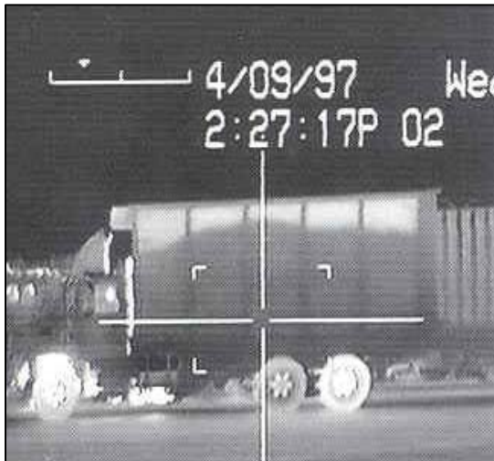
Figure 6: IRISystem Detecting Inoperable Brakes on the Vehicle
